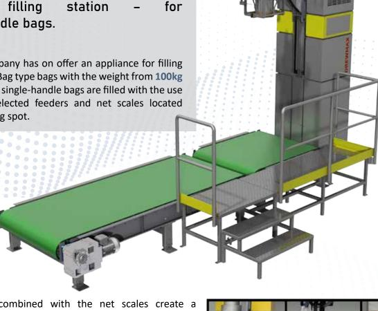
The filling line combined with the net scales create a semi-automatic packing appliance for loose / granulated / powdery products with the use of Big-Bag type bags.
