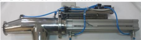
**PPR-01 chain conveyor** sampler – It is used mainly for granulated products.
