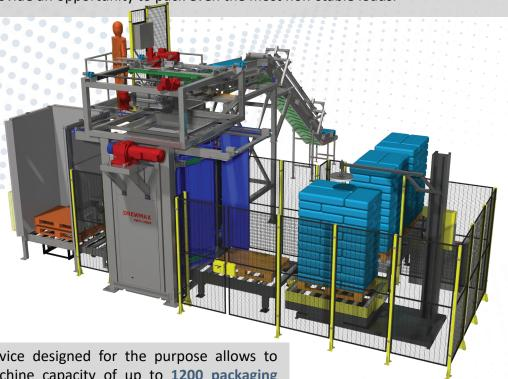
A gripping device designed for the purpose allows to reach the machine capacity of up to 1200 packaging products per hour. Dependent upon actual needs, the palletizer can be additionally equipped with a feeder of empty pallets and an accessory storage for spacers (cardboard or foil). Our scope of activity encompasses counselling, design, performance and service on the Customer's premises.
