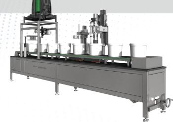
The feeder through which product is fed to a container is adjusted to the product qualities. It is possible to use the following types of feeders:
